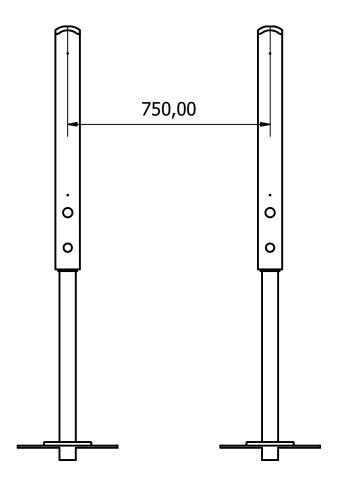
3. USING THE PILOT HOLES ON THE POSTS AS A GUIDE, SECURE THE PLAY PANEL TO THE POSTS USING THE FIXINGS PROVIDED.
