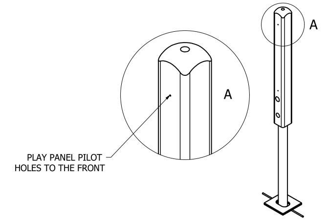
2. POSITION THE SECOND POST INTO THE FOUNDATION HOLE AS ILLUSTRATED BELOW.
