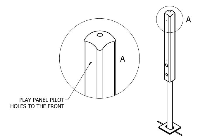
2. POSITION THE SECOND POST INTO THE FOUNDATION HOLE AS ILLUSTRATED BELOW.
