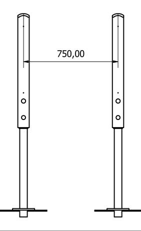
3. USING THE PILOT HOLES ON THE POSTS AS A GUIDE, SECURE THE PLAY PANEL TO THE POSTS USING THE FIXINGS PROVIDED.
