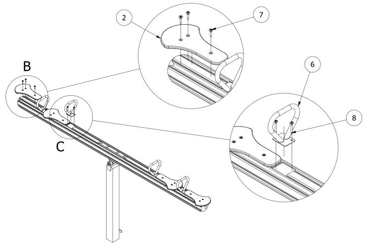
3. FINALLY, ENSURE UNIT IS LEVEL AND PLUMB, ALL FIXINGS HAVE BEEN TIGHTENED AND PROTECTIVE CAPS IN PLACE. ADD CONCRETE TO EACH FOUNDATION HOLE AND LEAVE FOR 48 HOURS
