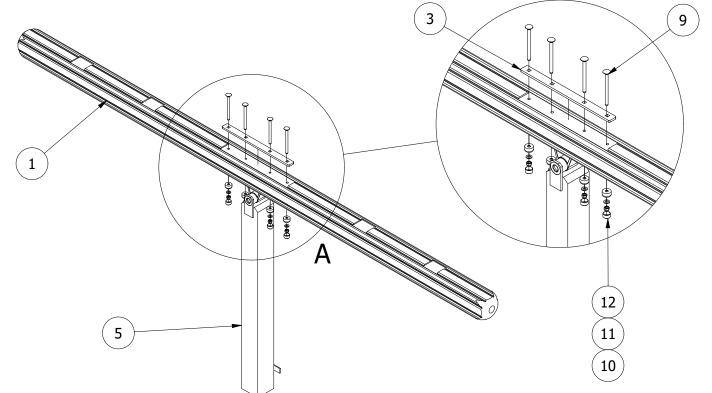
2. EACH HAND HOLE HAS A REBATE IN THE TIMBER TO AID THE LOCATION. INSERT THE HAND HOLD INTO THE REBATE AND SECURE USING THE SUPPLIED FIXINGS. POSITION THE SEAT BEHIND EACH HAND HOLD AND SECURE USING THE SUPPLIED FIXINGS.
