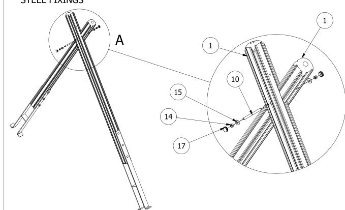
2. POSITION THE A-FRAMES INTO THE FOUNDATION HOLES AND BRACE. (TAKE NOTE OF THE POSITION OF THE POSTS AS SHOWN IN FIG 1) POSITION THE TOP BAR ONTO THE A-FRAMES AND SECURE IN PLACE.
