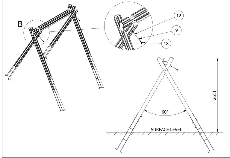
3. WITH BOTH FRAMES POSITIONED AND PROPPED IN THE FOUNDATION HOLES, POSITION THE MAIN SWING BEAM ONTO THE TOP A-FRAME BAR. USE THE SUPPLIED BOLTS TO SECURE.
