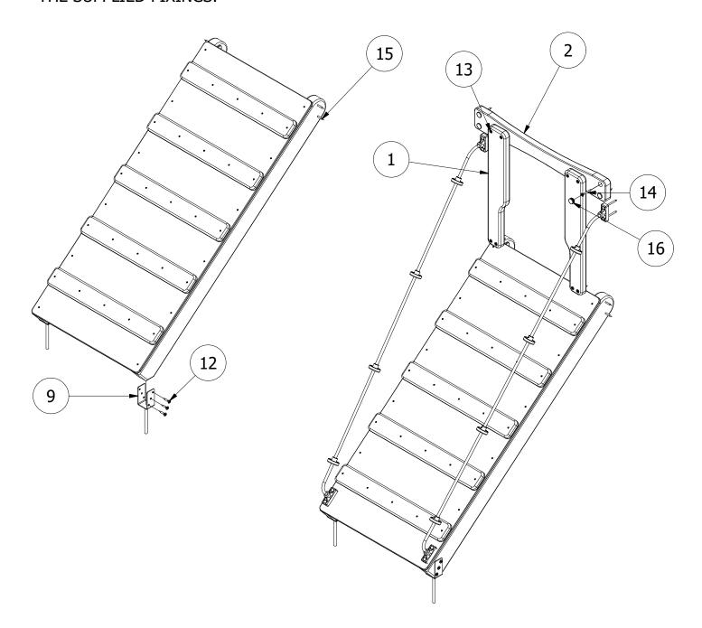
4. FINALLY, ENSURE UNIT IS LEVEL AND PLUMB, ALL FIXINGS HAVE BEEN TIGHTENED AND PROTECTIVE CAPS IN PLACE. ADD CONCRETE TO EACH FOUNDATION HOLE AND LEAVE FOR 48 HOURS
