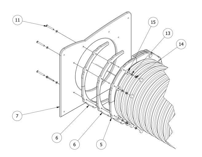
2. POSITION THE ASSEMBLED TUNNEL BETWEEN THE FOUNDATION HOLES. POSITION THE TIMBER POSTS ON THE INSODE OF THE PANEL. WHEN THE DESIRED POSITION HAS BEEN ACHIEVED, SECURE THE PANEL TO THE POSTS USING THE SUPPLIED SCREWS.
