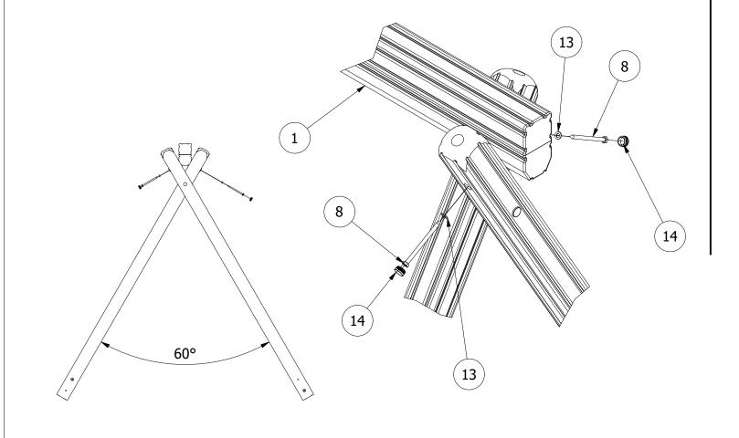
3. AS ILLUSTRATED, SECURE THE SWING HANGER TO THE UNDERSIDE OF THE TOP BAR
