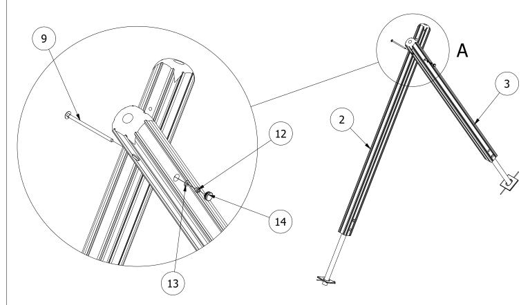
2. POSITION THE A-FRAMES INTO THE FOUNDATION HOLES AND BRACE. (TAKE NOTE OF THE POSITION OF THE POSTS AS SHOWN IN FIG 1) POSITION THE TOP BAR ONTO THE A-FRAMES AND SECURE IN PLACE.
