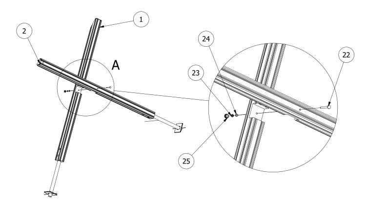
2. POSITION THE X-FRAMES INTO THE FOUNDATION HOLES AND BRACE. POSITION THE FRAMES TOGETHER AND SECURE USING THE SUPPLIED FIXING.
