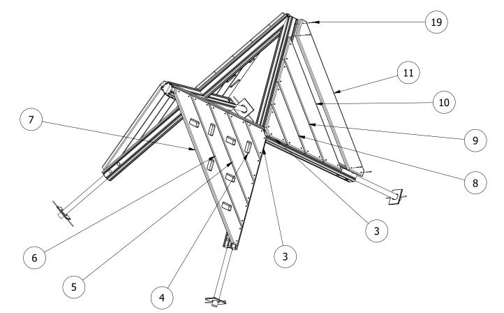
4. WITH RANDOM DISTRIBUTION, SECURE THE ROCK HOLDS TO THE BLANK PANELING ON BOTH SIDES.
