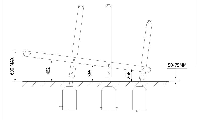
3. FINALLY, ENSURE UNIT IS LEVEL AND PLUMB, ALL FIXINGS HAVE BEEN TIGHTENED AND PROTECTIVE CAPS IN PLACE. ADD CONCRETE TO EACH FOUNDATION HOLE AND LEAVE FOR 48 HOURS
