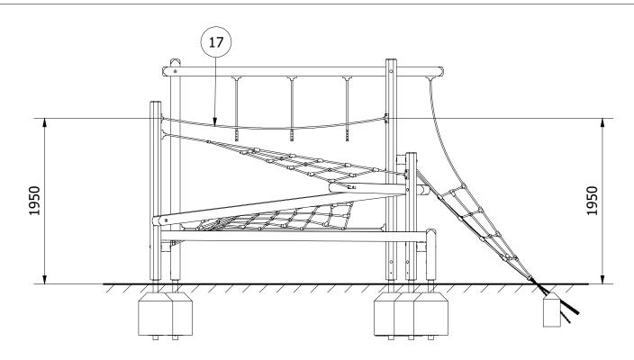
8. FINALLY, ENSURE THE UNIT IS LEVEL AND PLUMB. ALL FIXINGS HAVE BEEN TIGHTENED AND PROTECTIVE CAPS IN PLACE. ADD CONCRETE INTO THE FOUNDATIONS AND LEAVE 48 HOURS TO SET.
