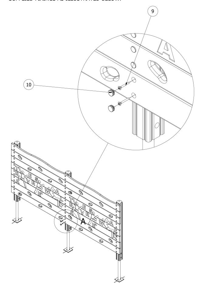
2. FINALLY, ENSURE UNIT IS LEVEL AND PLUMB, ALL FIXINGS HAVE BEEN TIGHTENED AND PROTECTIVE CAPS IN PLACE. ADD CONCRETE TO EACH FOUNDATION HOLE AND LEAVE FOR 48 HOURS
