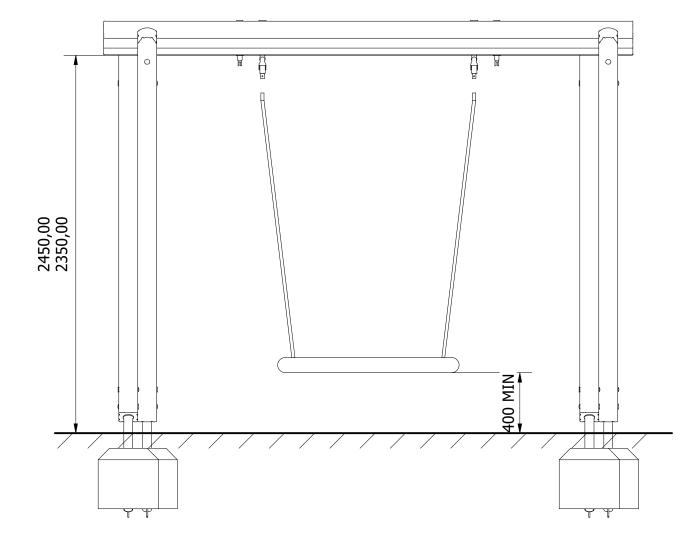
2. FINALLY, ENSURE UNIT IS LEVEL AND PLUMB, ALL FIXINGS HAVE BEEN TIGHTENED AND PROTECTIVE CAPS IN PLACE. ADD CONCRETE TO EACH FOUNDATION HOLE AND LEAVE FOR 48 HOURS
