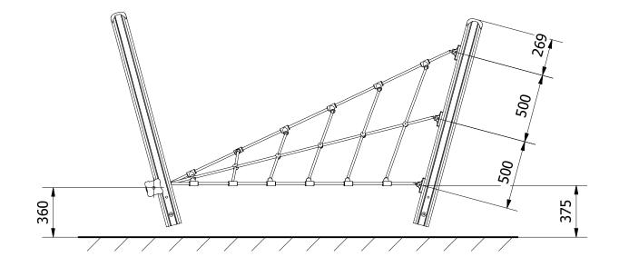
4. FINALLY, ENSURE ALL FIXINGS HAVE BEEN TIGHTENED AND PROTECTIVE CAPS IN PLACE. ADD CONCRETE TO EACH FOUNDATION HOLE AND LEAVE FOR 48 HOURS
