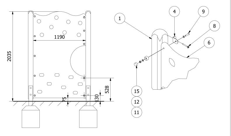
4. FINALLY, ENSURE THE UNIT IS LEVEL AND PLUMB, ALL FIXINGS HAVE BEEN TIGHTENED PROTECTIVE CAPS IN PLACE AND ROPE S TAUT. ADD CONCRETE TO EACH FOUNDATION HOLE AND LEAVE FOR 48 HOURS.
