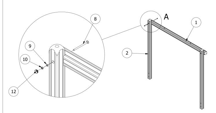
2. WITH THE MAIN FRAME IN PLACE, POSITION AND REMAINING POST INTO THE CENTRE OF THE UNIT. USE THE EYEBOLTS TO SECURE THE ROPE FROM THE TOP BAR, THEN ATTACH TO THE SIDE OF THE MAIN UPRIGHT, AND THE SIDE OF THE SMALLER STEPPING POST. **ENSURE ROPE IS TENSIONED**
