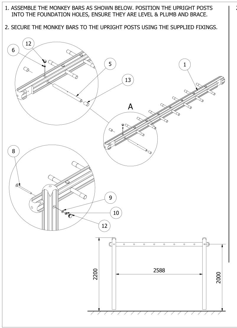
2. FINALLY, ENSURE UNIT IS LEVEL AND PLUMB, ALL FIXINGS HAVE BEEN TIGHTENED AND PROTECTIVE CAPS IN PLACE. ADD CONCRETE TO EACH FOUNDATION HOLE AND LEAVE FOR 48 HOURS
