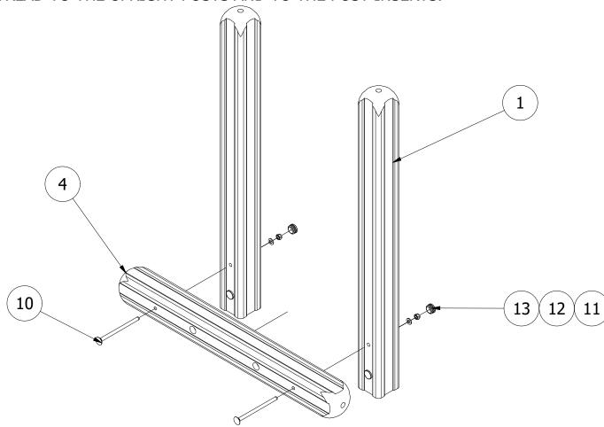
2. POSITION THE H-FRAMES INTO THE FOUNDATION HOLES AND SECURE THE SUPPORTING FRAME BRACES TO BOTH ENDS/ONE SIDE OF THE BRIDGE.
