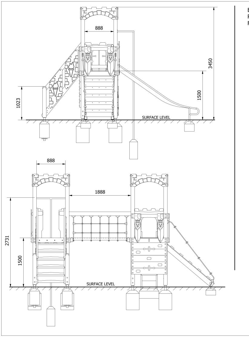
ENSURE UNIT IS LEVEL AND PLUMB, ALL FIXINGS HAVE BEEN TIGHTENED AND PROTECTIVE CAPS IN PLACE. ADD CONCRETE TO EACH FOUNDATION HOLE AND LEAVE FOR 48 HOURS.
