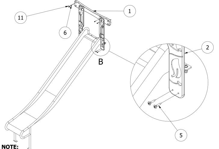
TO REDUCE THE RISK OF STEEL GALLING, USE LUBRICANT ON ALL STAINLESS STEEL FIXINGS
