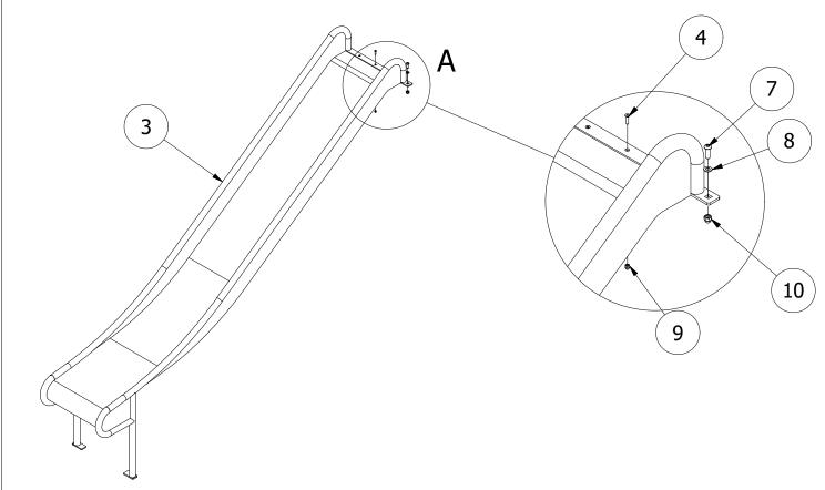
2. AS ILLUSTRATED, SECURE THE GUARDING SECTION AROUND THE SLIDE. ENSURE CRITICAL DIMENSIONS (FIG 1) ARE MAINTAINED.
