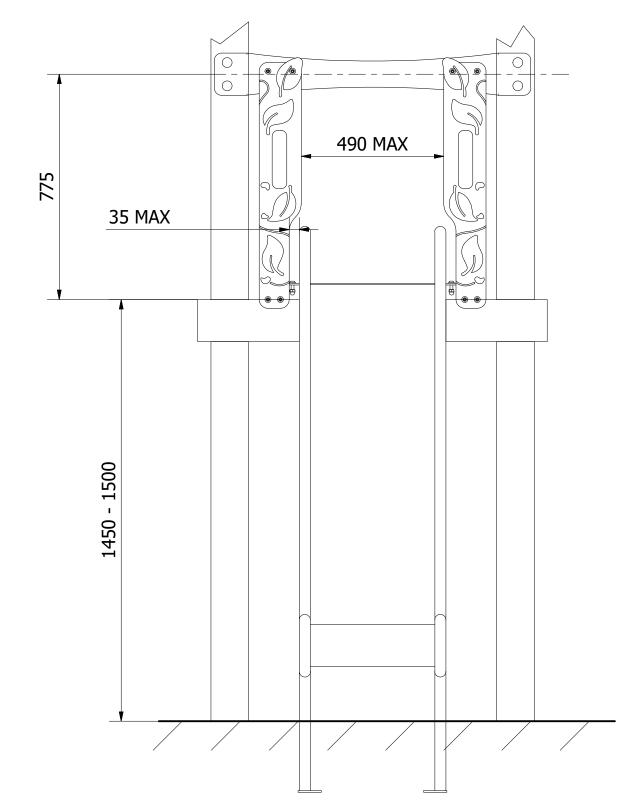
4. FINALLY, ENSURE UNIT IS LEVEL AND PLUMB, ALL FIXINGS HAVE BEEN TIGHTENED AND PROTECTIVE CAPS IN PLACE. ADD CONCRETE TO EACH FOUNDATION HOLE AND LEAVE FOR 48 HOURS
