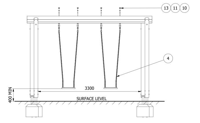
4. FINALLY, ENSURE UNIT IS LEVEL AND PLUMB, ALL FIXINGS HAVE BEEN TIGHTENED AND PROTECTIVE CAPS IN PLACE. ADD CONCRETE TO EACH FOUNDATION HOLE AND LEAVE FOR 48 HOURS
