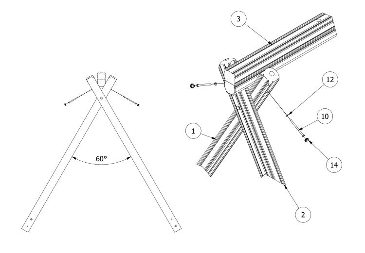
3. AS ILLUSTRATED, SECURE THE SWING HANGER TO THE UNDERSIDE OF THE TOP BAR NOTE: ENSURE THE SEAT SITS A MINIMUM OF 400MM FROM FINISHED SURFACE LEVEL TO UNDERSIDE OF THE SWING SEATS.
