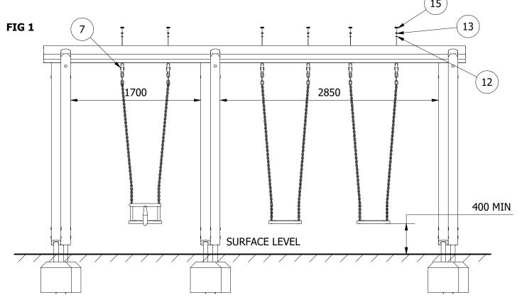
4. FINALLY, ENSURE UNIT IS LEVEL AND PLUMB, ALL FIXINGS HAVE BEEN TIGHTENED AND PROTECTIVE CAPS IN PLACE. ADD CONCRETE TO EACH FOUNDATION HOLE AND LEAVE FOR 48 HOURS
