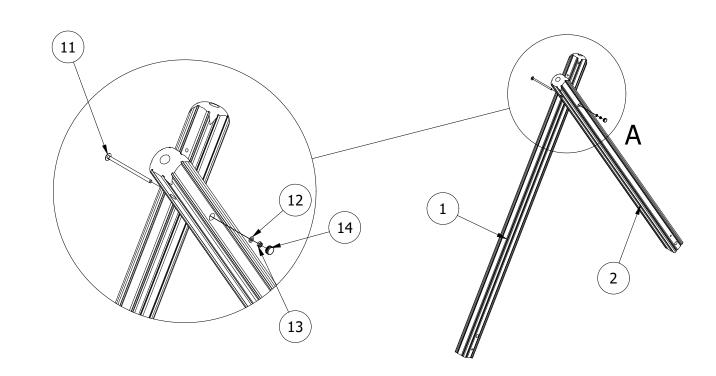
2. POSITION THE A-FRAMES INTO THE FOUNDATION HOLES AND BRACE. (TAKE NOTE OF THE POSITION OF THE POSTS AS SHOWN IN FIG 1) POSITION THE TOP BAR ONTO THE A-FRAMES AND SECURE IN PLACE.
