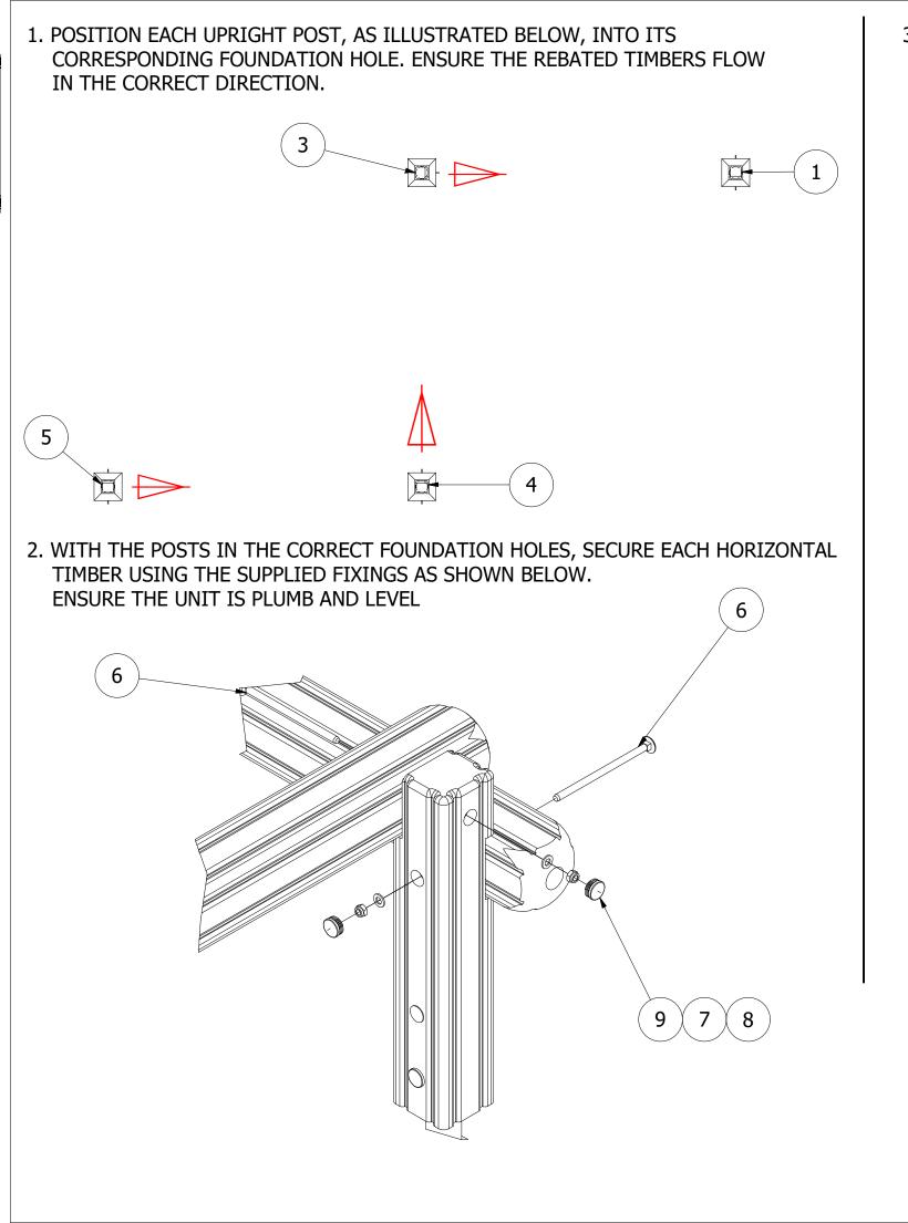
3. FINALLY, ENSURE UNIT IS LEVEL AND PLUMB, ALL FIXINGS HAVE BEEN TIGHTENED AND PROTECTIVE CAPS IN PLACE.
