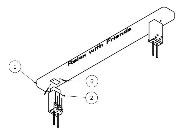
3. WITH THE LEGS SECURED TO THE BENCH TOP, PLACE THE BENCH INTO THE FOUNDATION HOLES.
