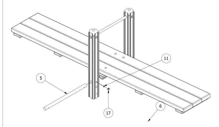
3. FINALLY, SECURE THE TWO HANDRAILS TO THE PIVOT BOARD. ENSURE ALL FIXINGS HAVE BEEN TIGHTENED AND PROTECTIVE CAPS IN PLACE.
