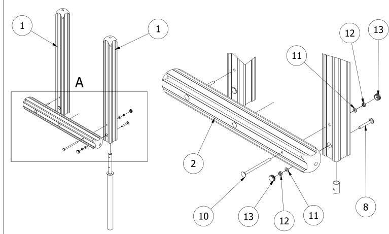
2. POSITION THE H-FRAMES INTO THE FOUNDATION HOLES AND SECURE THE SUPPORTING FRAME BRACES TO BOTH ENDS/ONE SIDE OF THE BRIDGE.
