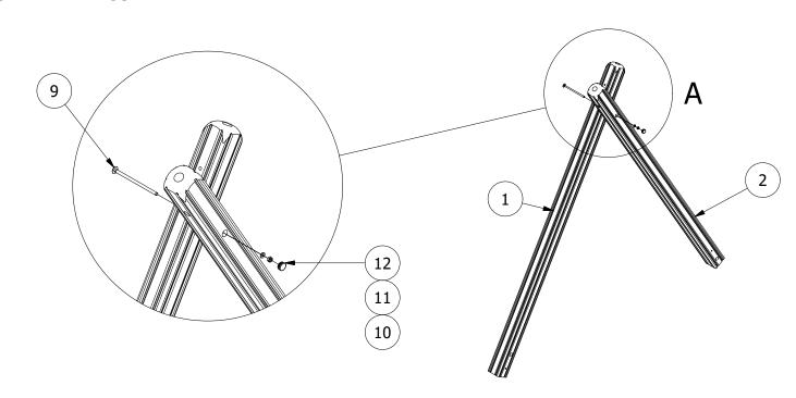
2. POSITION THE A-FRAMES INTO THE FOUNDATION HOLES AND BRACE. (TAKE NOTE OF THE POSITION OF THE POSTS AS SHOWN IN FIG 1) POSITION THE TOP BAR ONTO THE A-FRAMES AND SECURE IN PLACE.
