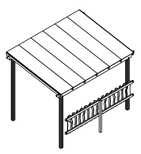
5. POSITION THE SIDE BARRIERS LEVEL WITH THE REAR BARRIER AND SECURE IN PLACE USING THE FIXINGS PROVIDED.
