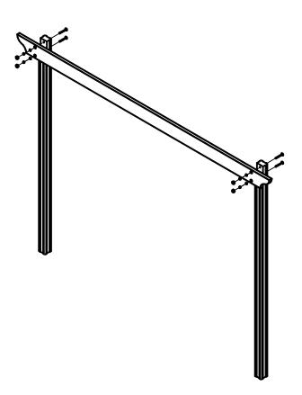
2. REPEATING STEP ONE CREAT THE SECOND FRAME AND POSITION INTO THE FOUNDATION HOLES.
