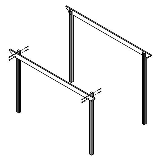
3. SECURE THE RAFTERS TO BOTH SIDES OF THE FRAME USING THE FIXINGS PROVIDED. RAFTER SPACINGS SHOWN ON PAGE 2.
