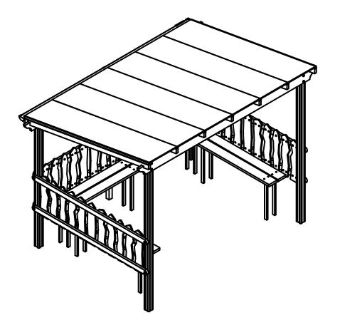
9. FINALLY, ENSURE THE UNIT IS LEVEL AND PLUMB, ALL FIXINGS HAVE BEEN TIGHTENED AND PROTECTIVE CAPS IN PLACE. ADD CONCRETE TO EACH FOUNDATION HOLE AND LEAVE FOR 48 HOURS.
