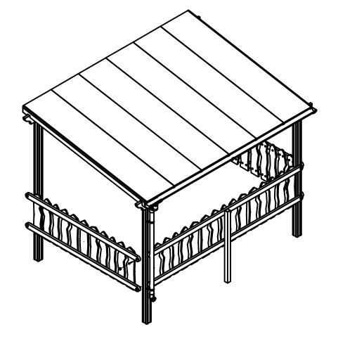
6. MOVE THE GUTTER CHANNEL INTO PLACE AND SECURE IN PLACE USING THE BRACKET AND FIXINGS PROVIDED.
