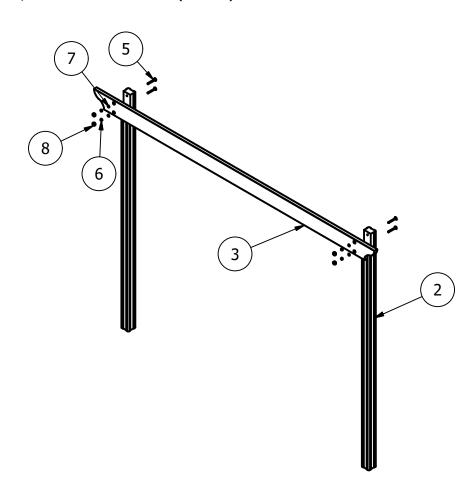
2. REPEATING STEP ONE CREATE THE REAR (SMALL) FRAME AND POSITION INTO THE FOUNDATION HOLES.
