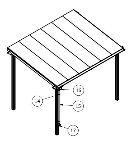
5. FINALLY. ENSURE THE UNIT IS LEVEL AND PLUMB, ALL FIXINGS HAVE BEEN TIGHTENED AND PROTECTIVE CAPS IN PLACE. ADD CONCRETE TO EACH FOUNDATION HOLE AND LEAVE FOR 48 HOURS.
