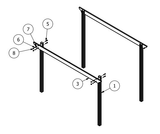
3. SECURE THE RAFTERS TO BOTH SIDES OF THE FRAME USING THE FIXINGS PROVIDED. RAFTER SPACINGS SHOWN ON PAGE 2.
