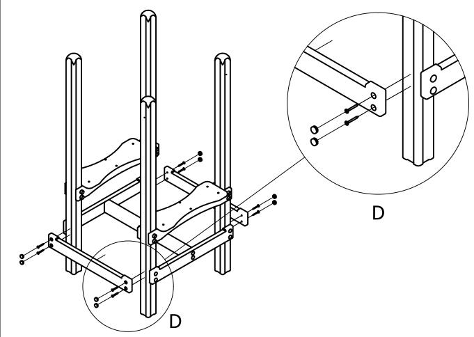
7. POSITION THE DECK AS ILLUSTRATED BELOW AND SECURE WITH THE FIXINGS PROVIDED.
