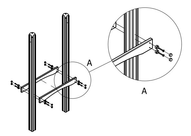
2. USING THE FIXINGS PROVIDED SECURE THE HDPE BENCH TOPS TO THE BENCH SUPPORTS AS ILLUSTRATED BELOW.
