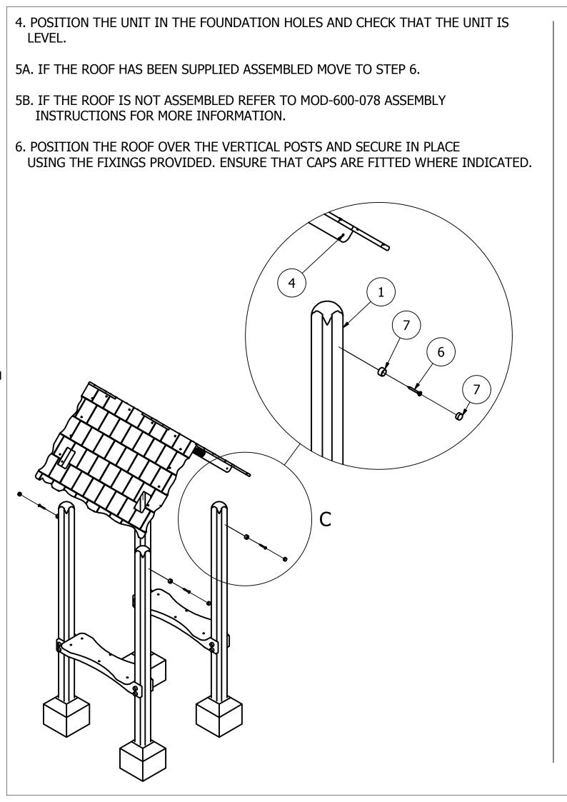
7. ENSURE THE UNIT IS LEVEL AND PLUMB, ALL FIXINGS HAVE BEEN TIGHTENED AND PROTECTIVE CAPS ARE IN PLACE. ADD CONCRETE TO EACH FOUNDATION HOLE AND LEAVE FOR 48 HOURS. ONCE THE CONCRETE HAS BEEN ADDED LEAVE FOR 48 HOURS.
