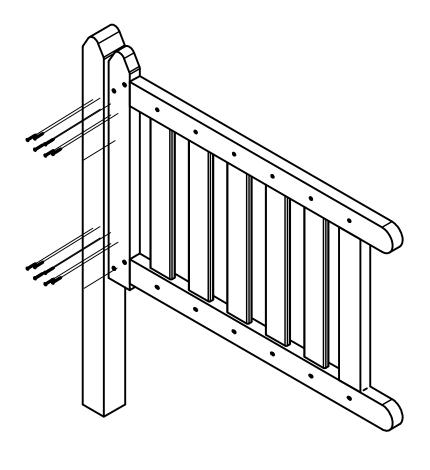
3. ONCE THE GATE IS SECURED TO THE POST AND ABLE TO OPEN AND CLOSE FREELY, SECURE THE RUBBER BUMPERS TO THE POST WHERE THE GATE CLOSES TO. ENSURE THAT THE FIXINGS ARE NOT PROUD AND THE GATE ONLY CONTACTS THE RUBBER.
