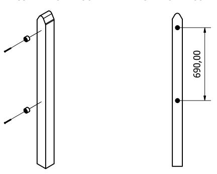
4. FINALLY, ENSURE UNIT IS LEVEL AND PLUMB, ALL FIXINGS HAVE BEEN TIGHTENED AND PROTECTIVE CAPS IN PLACE. ADD CONCRETE TO EACH FOUNDATION HOLE AND LEAVE FOR 48 HOURS
