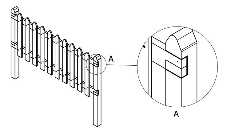
3. WITH THE FENCE PANEL CORRECTLY PLACED SECURE THE PANEL USING THE POST PALES AND FIXINGS PROVIDED. ENSURE THAT THE POSTS STAY IN POSITION WHILE THE PANEL IS BEING SECURED.
