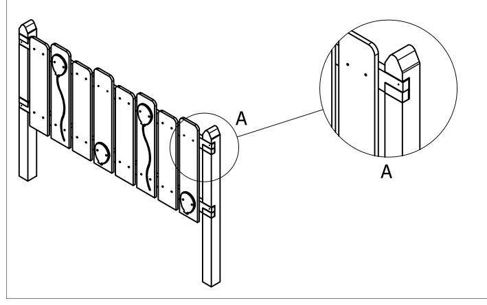
3. WITH THE FENCE PANEL CORRECTLY PLACED SECURE THE PANEL USING THE POST PALES AND FIXINGS PROVIDED. ENSURE THAT THE POSTS STAY IN POSITION WHILE THE PANEL IS BEING SECURED.
