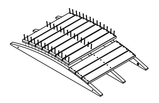
2. POSTITION THE VERTICAL POSTS AGAINST THE BASE AND SECURE USING THE FIXINGS SUPPLIED
