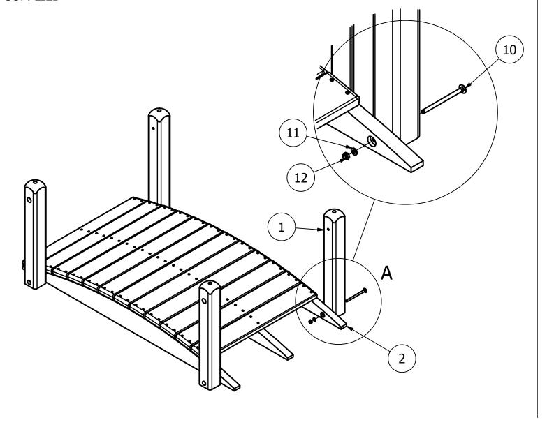
3. AS ILLUSTRATED, SECURE THE THE ARCHED HAND RAIL TO THE VERTICAL POSTS
