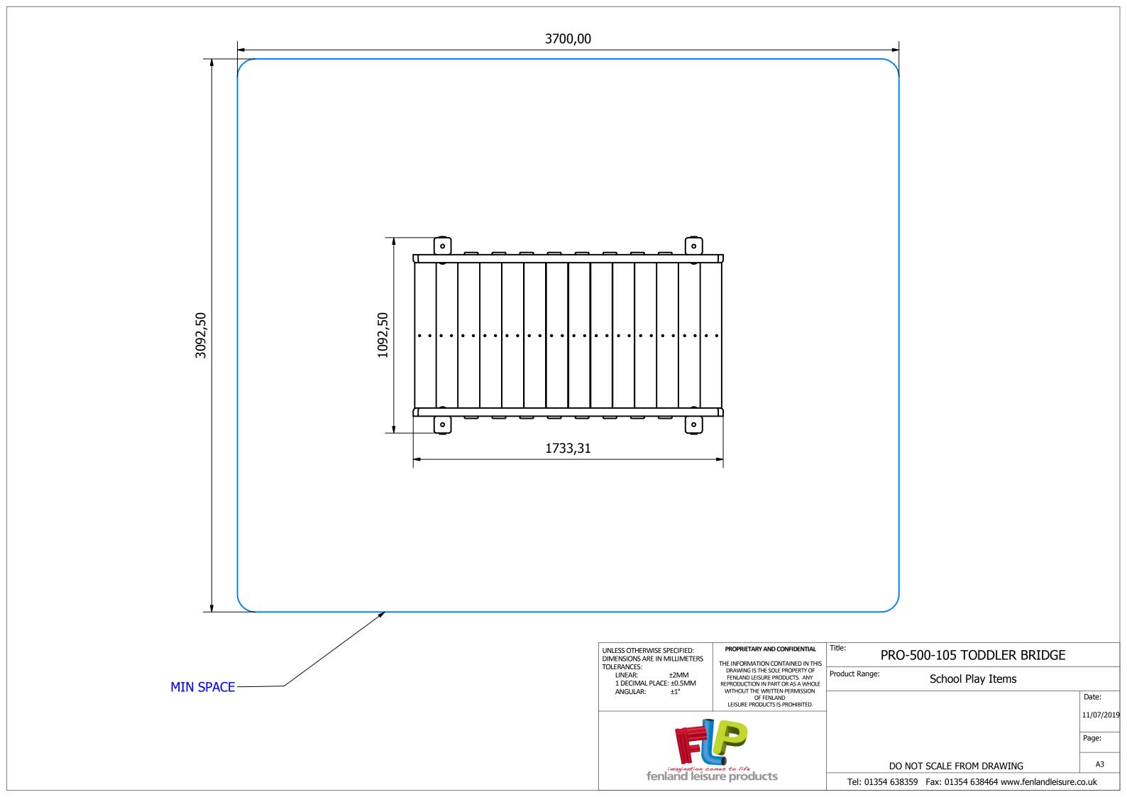
CREATE THE BASE AS SHOWN BELOW USING THE SUPPLIED FIXINGS. ENSURE THAT THE LAST TWO DECKING TIMBERS ON BOTH SIDES ARE NOT ATTACHED TO ALLOW ACCESS TO THE INTERNAL FIXING POINTS.
