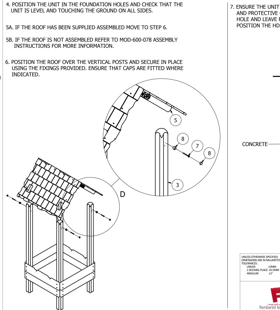
7. ENSURE THE UNIT IS LEVEL AND PLUMB, ALL FIXINGS HAVE BEEN TIGHTENED AND PROTECTIVE CAPS ARE IN PLACE. ADD CONCRETE TO EACH FOUNDATION HOLE AND LEAVE FOR 48 HOURS. ONCE THE CONCRETE HAS BEEN ADDED POSITION THE HDPE COVER OVER THE BASE AND LEAVE FOR 48 HOURS.
