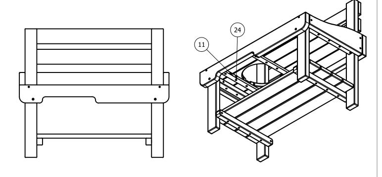
7. REMOVE THE OP BACK PANEL AND POSITION THE SHELF AS ILLUSTRATED BELOW. SECURE THE SHELF USING THE FIXINGS PROVIDED AND THEN RECONNECT THE TOP BACK PANEL.
