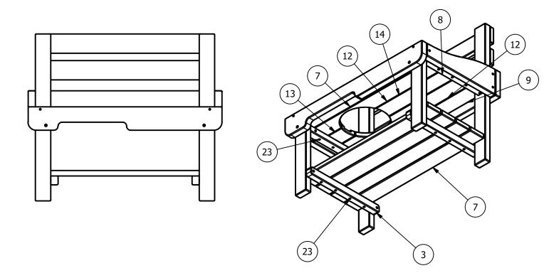
6. WITH THE COUNTER TOP TIMBERS SECURED IN POSITION, SECURE THE SINK BRACES AS SHOWN BELOW.
