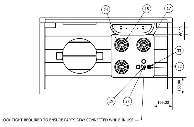
10. POSITION THE HDPE NUMBER SLIDER ON THE FRONT PANEL AS SHOWN BELOW AND SECURE USING THE FIXINGS PROVIDED.
