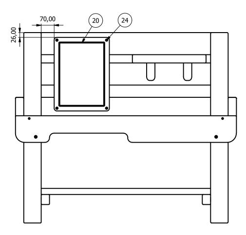
9. POSITION THE HOB AS SHOWN BELOW AND SECURE USING THE FIXINGS PROVIDED. ENSURE THE HOB KNOB FIXINGS HAVE ENOUGH SPACE BEHIND THE HDPE PANEL. A COUNTER BOAR HOLE MAY BE REQUIRED.
