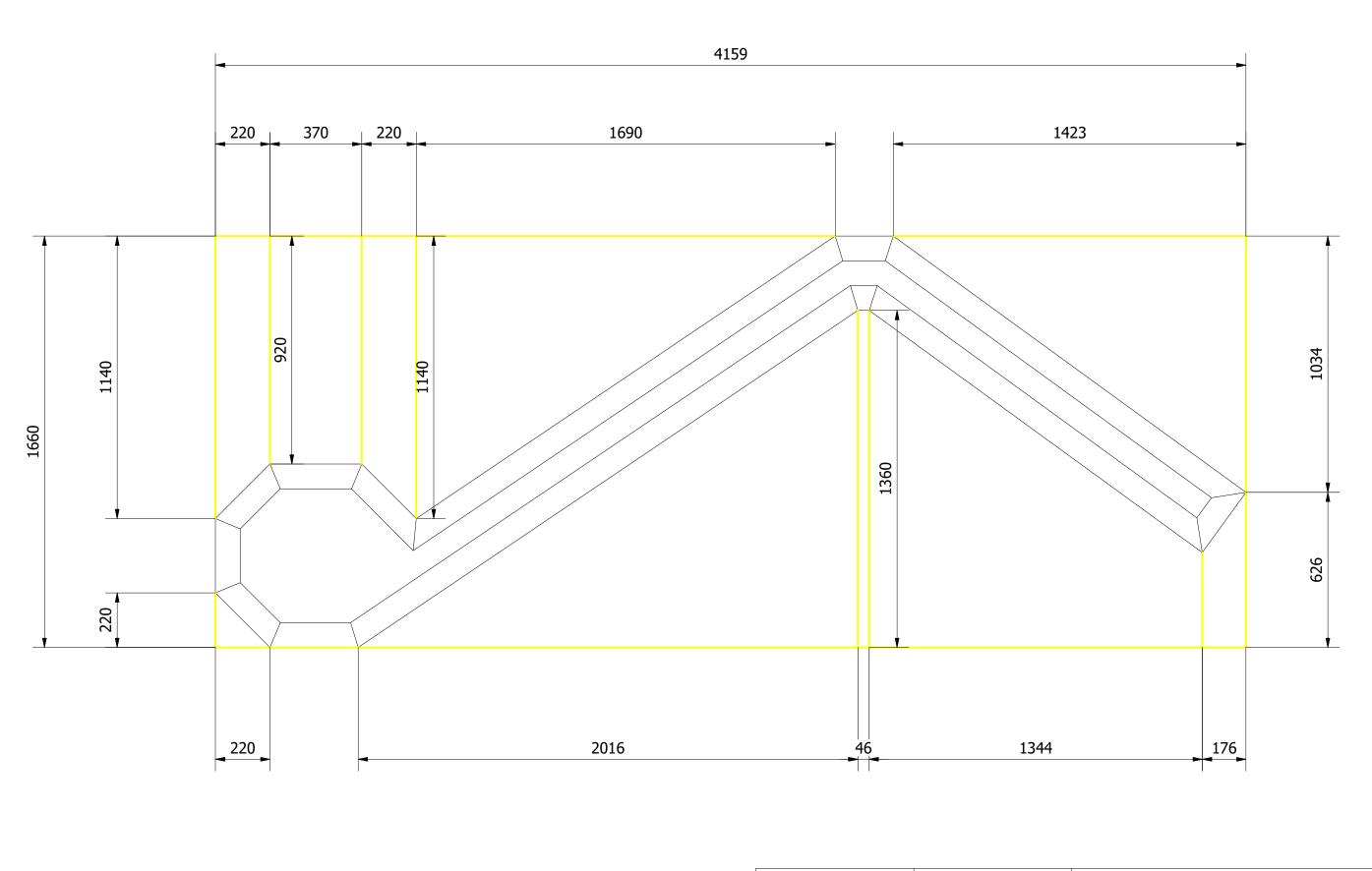
PROPRIETARY AND CONFIDENTIAL PRO-500-223 STEPPING SNAKE (TT20) THE INFORMATION CONTAINED IN THIS DRAWING IS THE SOLE PROPERTY OF FENLAND LEISURE PRODUCTS. ANY REPRODUCTION IN PART OR AS A WHOLE WITHOUT THE WRITTEN PERMISSION OF FENLAND LEISURE PRODUCTS IS PROHIBITED. LINEAR: ±2MM 1 DECIMAL PLACE: ±0.5MM ANGULAR: ±1° Product Range: FITNESS TRAIL DO NOT SCALE FROM DRAWING
