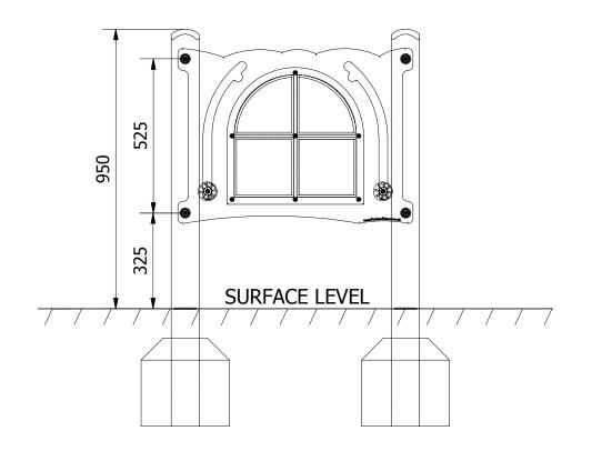
4. FINALLY, ENSURE ALL FIXINGS HAVE BEEN TIGHTENED AND PROTECTIVE CAPS IN PLACE. ADD CONCRETE TO EACH FOUNDATION HOLE AND LEAVE FOR 48 HOURS
