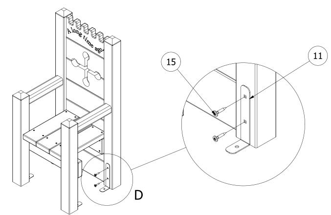
5. MARK THE POSITION OF THE HOLES AND DRILL A Ø12 X 130 DEEP HOLE INTO THE LEVEL CONCRETE BASE. INSERT THE GROUND ANCHOR AND REPLACE THE UNIT OVER THE HOLES. SECURE IN PLACE USING A M12 X 120 HEX HEAD BOLT.
