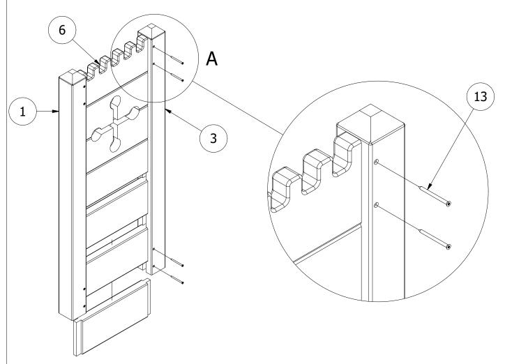
2. USING THE MORTICE AND TENON, INSERT THE ARMS INTO THE LARGER UPRIGHT POSTS (ITEM 1 & 3) AND INTO THE ARM UPRIGHT POSTS (ITEM 2).
