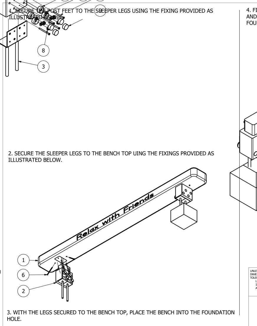
4. FINALLY, ENSURE UNIT IS LEVEL AND PLUMB, ALL FIXINGS HAVE BEEN TIGHTENED AND ANY PROTECTIVE CAPS NEEDED ARE IN PLACE. ADD CONCRETE TO EACH FOUNDATION HOLE AND LEAVE FOR 48 HOURS.
