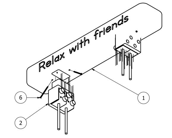
3. WITH THE LEGS SECURED TO THE BENCH TOP, PLACE THE BENCH INTO THE FOUNDATION HOLES
