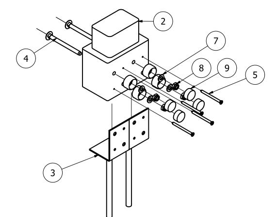
2. SECURE THE SLEEPER LEGS TO THE BENCH TOP UING THE FIXINGS PROVIDED AS ILLUSTRATED BELOW.
